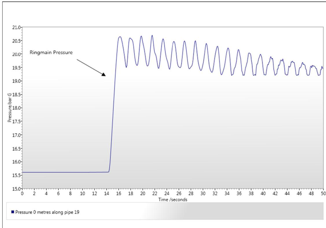
As can be seen, not only has the maximum pressure fluctuation reduced to around 1 Bar, the fluctuation itself decreases over time. This was deemed acceptable
