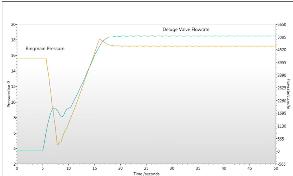
What can be seen here is a large drop in ringmain pressure, resulting in a small drop in deluge valve flowrate around the 10 s mark. The pressure drop, although large, is fairly gradual and therefore this does not impact upon the performance of the network.
